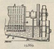
ing the parts forming said machines or apparatus so that the sand and other matter adhering to castings coming from the sand mould on being treated thereby are entirely removed therefrom, and received by receptacles from which such sand or refuse can be easily discharged.
