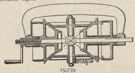
Tube Scrapers.—S. M. Cockburn, J. R. Temperley, and J. Temperley, London.—9,246.—This invention relates to a contrivance for breaking and removing the incrustation which adheres to the interior surface of tubes, particularly the tubes of water-tube boilers, a, a are two scaling tools oppositely pivoted on a socket c.
