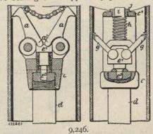
which is secured to a tubular arm d, which contains the mechanism of a pneumatic hammer and serves as a medium for the conveyance of energy by fluid under pressure and as means for manipulating the tool and causing it to effect the desired result at every part of the internal surface of the tube.
