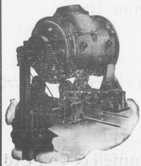
Since the introduction in America of the Bessemer Process for refining copper matte the Allis-Chalmers Co. has, with but few exceptions, furnished all the Converters used by the smelters in the
