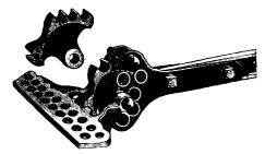
S simple and strong, and is capable of many adjustments to suit any line of draught desired.
