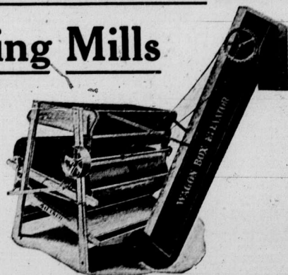
This cut shows a No. 3 40-in. Mill with Wagon Box Elevator. Capacity, 75 to 100 bushels per hour.
