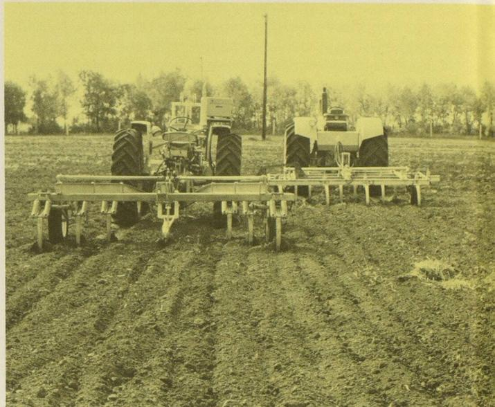
The operator drives the master tractor (right) while the slave tractor follows behind and to one side, doubling the amount of work done. The tractors, both pulling cultivators, are linked by a cable through which electronic signals automatically control the speed and steering of the slave vehicle.
