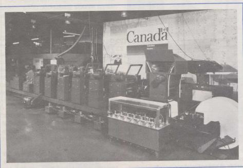
This variable size press from Sanden Machine Limited of Cambridge, Ontario requires only a pull on a lever to make it the fastest available today for size changeover.
