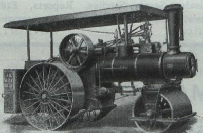
CASE 8 1/4 x 10 Inch Cylinder 10-Ton Road Roller
