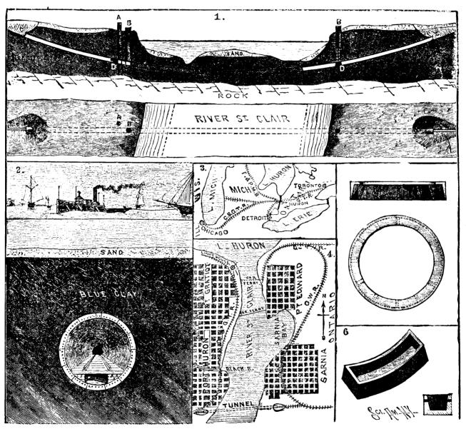
Sectional elevation and plan of tunnel; A, pump shaft; B, brick air shafts; C, cuttings; DD, bulkheads.
