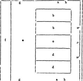
The entire building is 20x25 feet. b b are wheat bins, rye or barley bins, d d are oat bins , around these bins is an open space or walk, a, a, a, 20 inches wide; e is the bottom; g g are doors, h h h windows,
