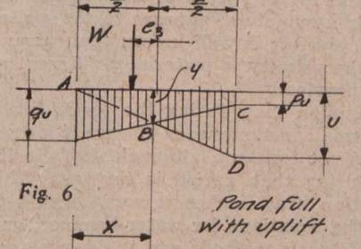
How the uplift can be regarded as producing an overturning moment, and at the same time the counter-moment of the foundation reaction be wilfully neglected, is beyond the writer's comprehension. It is a case of mechanics, pure and simple.
