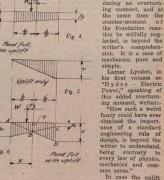
lbs. per sq. ft. and the upward water pressure is only capable of exerting 1,000 lbs. per sq. ft., it is evident that the foundation reaction still in contact with the base of the block, must exert 2,000 lbs. per sq. ft. By increasing the uplift to 3,000 lbs. per sq. ft., the block will be entirely sustained by the intervention of the state of the block will be entirely sustained by the intervention. L d interposed film of water between base of block and its
