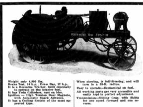
When plowing, is Self-Steering, and will turn in a 25-ft. radius. Easy to operate---Economical on fuel. All working parts are very accessible and easily kept in perfect adjustment. Transmission---Siding Gear, with Shifts for one speed forward and one re-verse.
