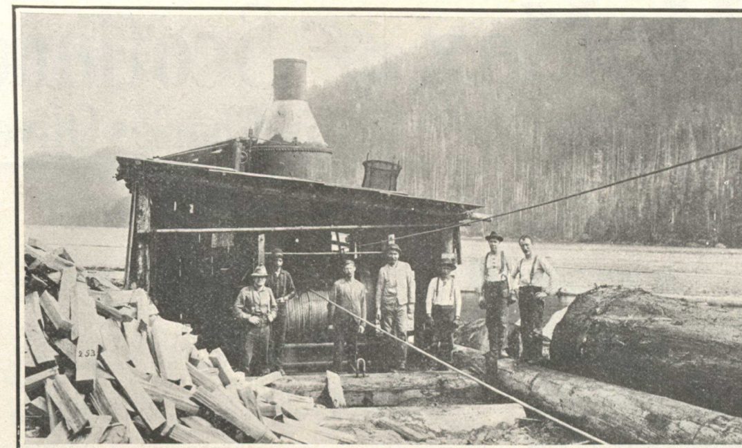
Hauling logs over a road to the water. This used to be done by horses, but donkey engines are now used. The lower heavy cable will be from one to two miles long. The lighter cable is to draw back the heavy cable when the logs have reached the engine.
