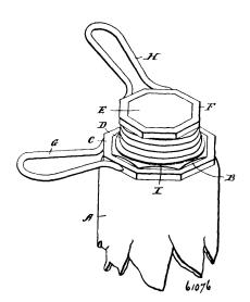
neck thereof, a threaded cover adapted to run upon the neck, a polygonal shaped top formed with the cover, and two wrenches adapted to fit the shoulder and top, as specified.
