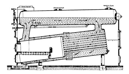
A Mumford internally fired boiler requires from 10 to 25 per cent. less fuel than a return tubular boiler.
