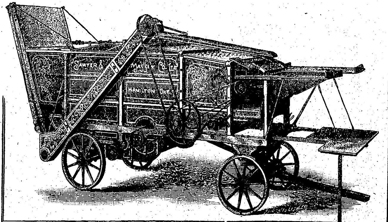
Belt Side View of the "Peerless" Thresher, showing Elevator and Straw Stackers folded.
