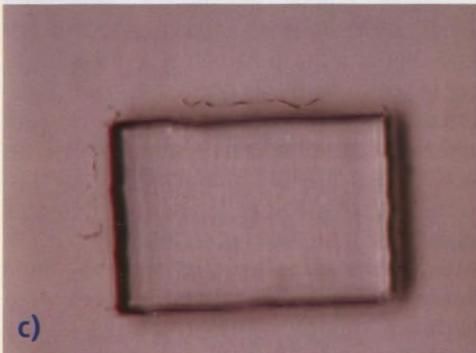
▲ Ablation experiments with germanium-doped silica glass on silicon wafers: Comparative irradiation at 193 nm and 157 nm
