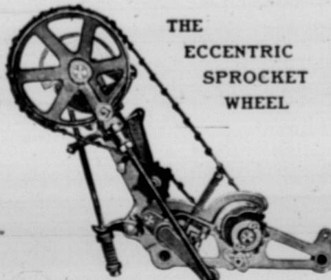
**N**OTICE that three of the arms of the Sprocket Wheel are shorter than the other three which accounts for greater power and speedier work.
