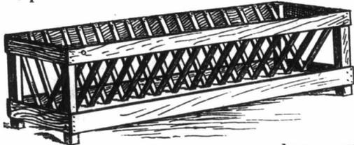
haps give you, as also your many readers, a more correct idea of how the rack is constructed. It will be noticed that around the bottom there is a trough three inches deep for roots, grain, etc., and to catch bits of the hay that break off.
