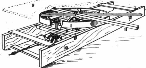
which is on the end of the tumbling or driving rod of the horse power. No. 7 is a brace, and on it is fastened a roller which rides on pinion 4 holding it down in place. No. 8 is a brace, which holds the bottom boxing of drive wheel axle. No. 10 is the frame, 10 inches high. The arm, 11, is ten feet long, and to it the horse is hitched. No. 12 is also ten feet long, and to it the horse is tied. No. 9 represents the cover for the power.
