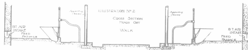
Showing two rows of cow stalls and relative positions of galvanized steel stalls, columns, mangers, water bowls, passages and gutters.
