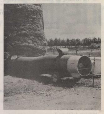
45-foot "I" beams. It can be raised or lowered by winches. The dried hay can be left in the tower through the winter. An oil-fired dryer forces warm air into the centre of the tower (upper right); the air passes out through the hay, carrying the moisture with it. The bung is taken from the roof and the double auger reversed to move the hay into the centre of the tower to drop down to the bottom duct. A conveyor through the side catches the hay and moves it out (lower left).
