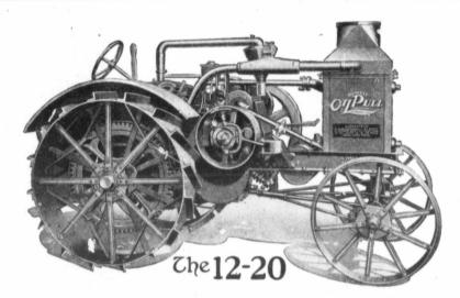
Capacity - Pulls three plows - operates 22-inch thresher.
