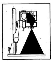
does not go straight from lamp to negative, but is deflected downwards by a mirror. Heat escapes not only through lamphouse vents but also from back of mirror. Lamp may be raised and lowered, as well as rotated to ensure precise centering with mirror. Illumination is totally even, yet retains the crispness of a condensor enlarger.
