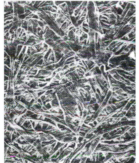
The surface of writing paper looks like this when magnified 220 times. Wood fibres, now flattened into tiny ribbons, overlap each other in all directions.
