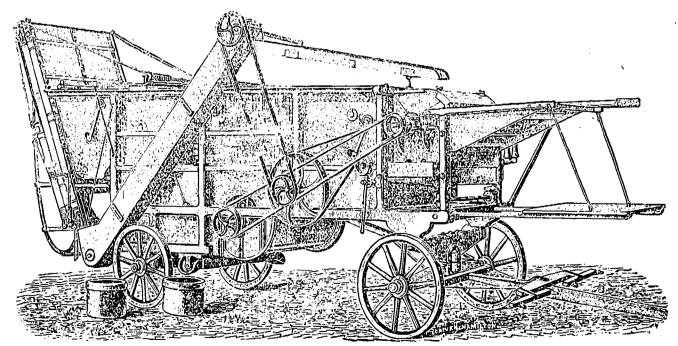
Belt Side View of the "Peerless," showing Elevator and Straw Stacker folded.
