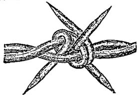
Four-Point Barb Galvanized steel Wire Fencing.
