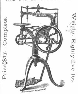
This is the best Saw made has 18 in. swing, ents 14 thick down to thin veneer, will do inlaying without tilting the table, it cuts so true.
