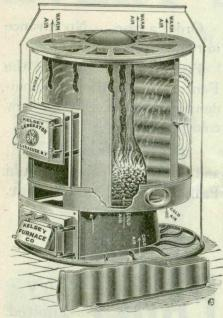
Note Carefully :-Formation of Fire Pot, Large Heating Surface, Great Air Capacity.
