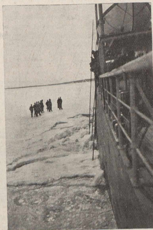
Fig. 6.—The "Montcalm" stuck for 10 hours in the ice below the Richelieu Rapids. Observe the effect of the circulating water in removing the frazil.
