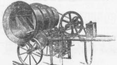
either continuously or in batches, and can be operated either by Hand, Steam or Gasoline Power.
