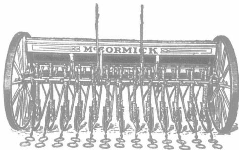
McCormick drills have one very important feature. The disk bearings turn easily and are as nearly dust proof as it is possible to make disk bearings. Only clean oil reaches them, and that from the inside, tending to keep out all dust and grit, and keeping the bearings free-running.
