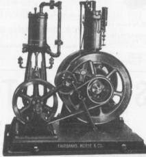
This arrangement is most convenient and economical in small sizes where the Compressor and Engine must occupy a minimum space.
