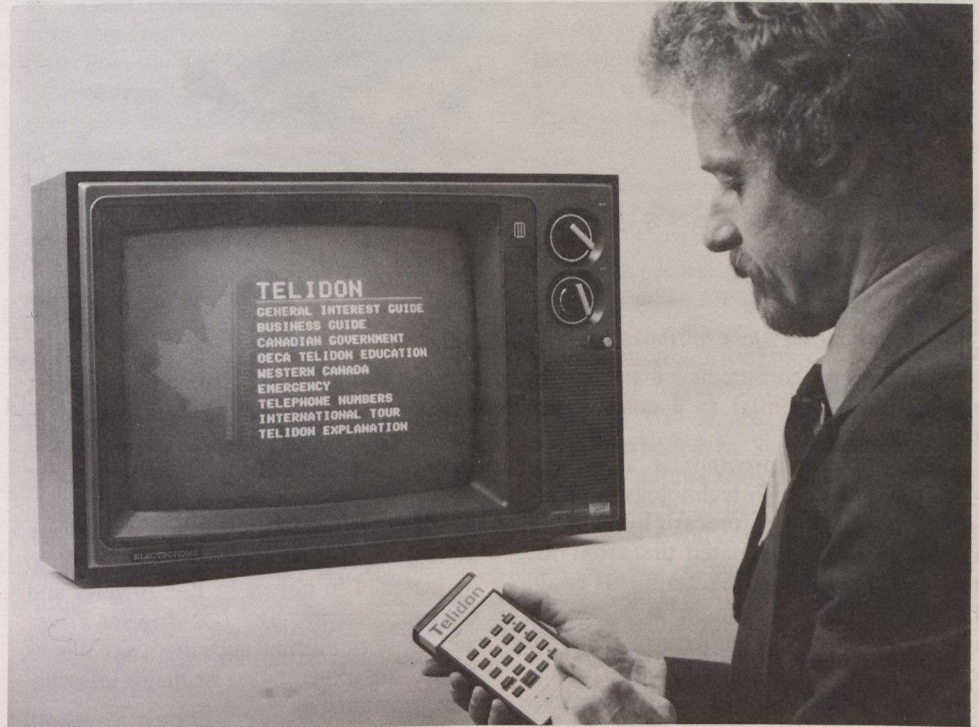
Telidon users can retrieve or insert information with calculator-like unit.
