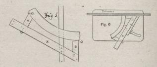
times fastened by two wood-screws from the back of the gauge, which is set at an angle of 60 degrees, and by others is attached to the table by two iron dowel pins, but the safest way is to use the two dowels in the table and one screw through the back of the gauge.
