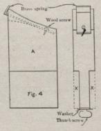
care being taken that the angle is right for the required number to the circle, viz., 90 degrees for four and 45 degrees for eight, etc.
