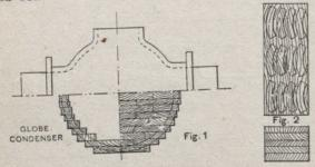
Fig. 2 illustrates the method of sawing several segments of the same dimensions in one operation, the number being determined by the thickness of the stock, the limit of the saw and the patternmaker's judgment. They are now ready to be jointed and this is the point I wish to emphasize in this article.
