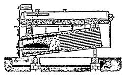
The Mumford Standard boiler is internally fired and no heat is wasted by radiation as in an externally fired boiler.
