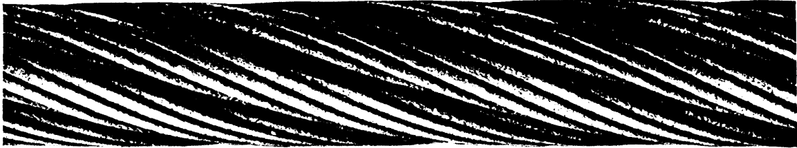
Illustration of Winding Rope, 240 fms. long x 3½ circ. Galvanized Special Improved Patent Steel. Compound Make, supplied to Kenneil Collieries, Bo'ness, Scot., which gave a record life of 6 years and 2 months. Showing condition when taken off.
