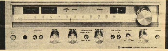
SX-780 continuous power output of 45 watts per channel, into 8 ohms, from 20 to 20,000 Hz, with no more than 0.05% total harmonic distortion. In addition to all of the above features, this model also includes; Pioneer DC Direct-Coupled Power Amplifier Circuitry, Musicality preserved in PHONO EQ, Low Cut Filter, Tape-Dubbing—Deck 1 to Deck 2 in Stereo.
