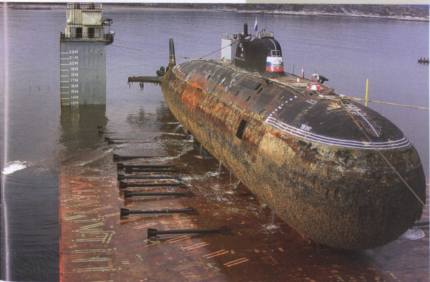
Dismantling a nuclear submarine entails 13 phases including transportation to the shipyard, reactor defuelling, placement in a dry dock, dismantlement, storage and transport of the spent nuclear fuel.
