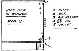
METHOD OF VENTILATING WINDOWS TO PREVENT FROSTING OF GLASS.
