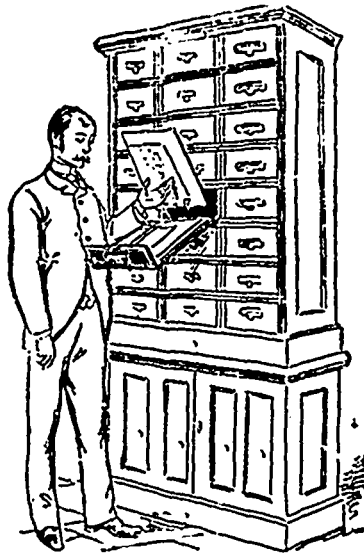
Shannon Filing Cabinet on base, showing how papers may be examined without removing drawer.
