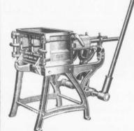
Their rapidity of operation produces building blocks at the lowest possible cost. Embody the only principle (face down) permitting the practical use of rich facing material with less expensive material in back of blocks.
