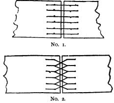
Cut No. 1 represents the right side of a belt, or the side running next the pulley, while cut No. 2 represents the reverse side of the same belt. On the right side the lacings are double between the two inside rows of holes, while a
