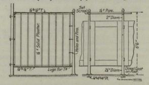
fixed with a set screw at every post. The frame reaches to within 10 inches of the floor and is covered with wire lath, not shown in the sketch. Where the frame meets the wall, the plaster is curved out so as to cover the steel shapes and form a good-looking junction
