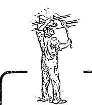
Saves all the trouble of taking down the pipe and threading it at the work-bench.
