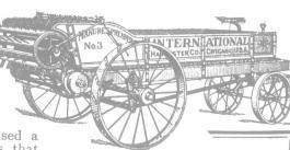
having a vibrating rake in front of the beater or cylinder which levels the load as it passes backward toward the spreading mechanism.
