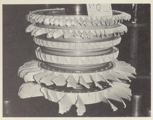
Destruction caused to the compressor rotors of a turboprop aircraft engine which ingested two pigeons.
