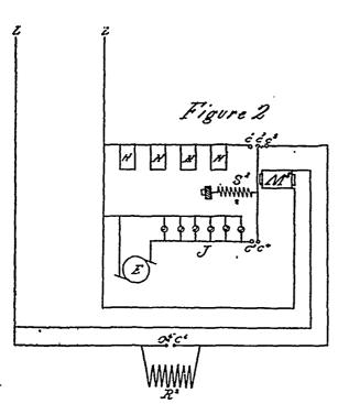
The manner in which this automatic switch and storage arrangement works is as follows: Arrange a two-throw hand switch for the purpose of turning on and off the power or lights in such a way that whenever the switch is turned one way it will connect C<sup>3</sup> with C<sup>4</sup>.
