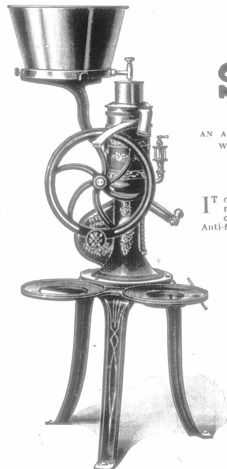
"NATIONAL" NO. 1 HAND POWER. Capacity, 330 to 350 lbs. per hour.
