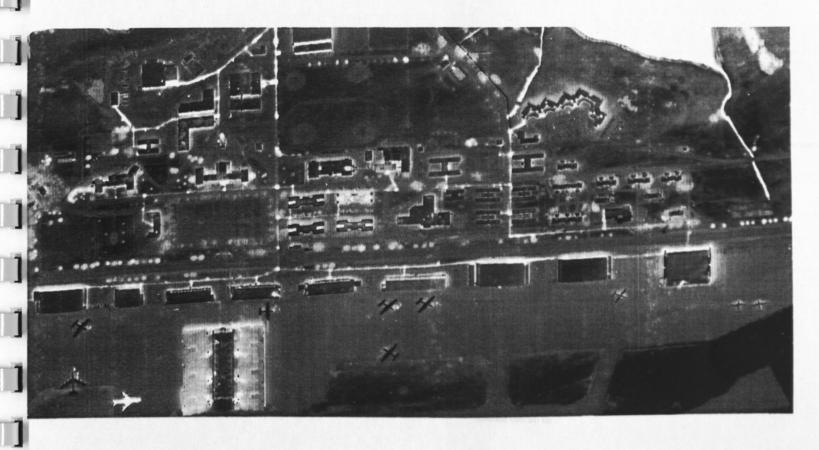
Figure 15. Thermal infrared linescan image of an airport. White is "hot" and black is "cold" in this image. The image was taken at night. Notice the "hot" buried steamlines and trees along the roadsides. Warm auxillary power units (APU's) can be seen near some of the aircraft. One aircraft appears anomalously warm compared to the others. It may have been parked inside the nearby hangar not long before the image was acquired. (Courtesy of Intera Technologies Ltd.)
