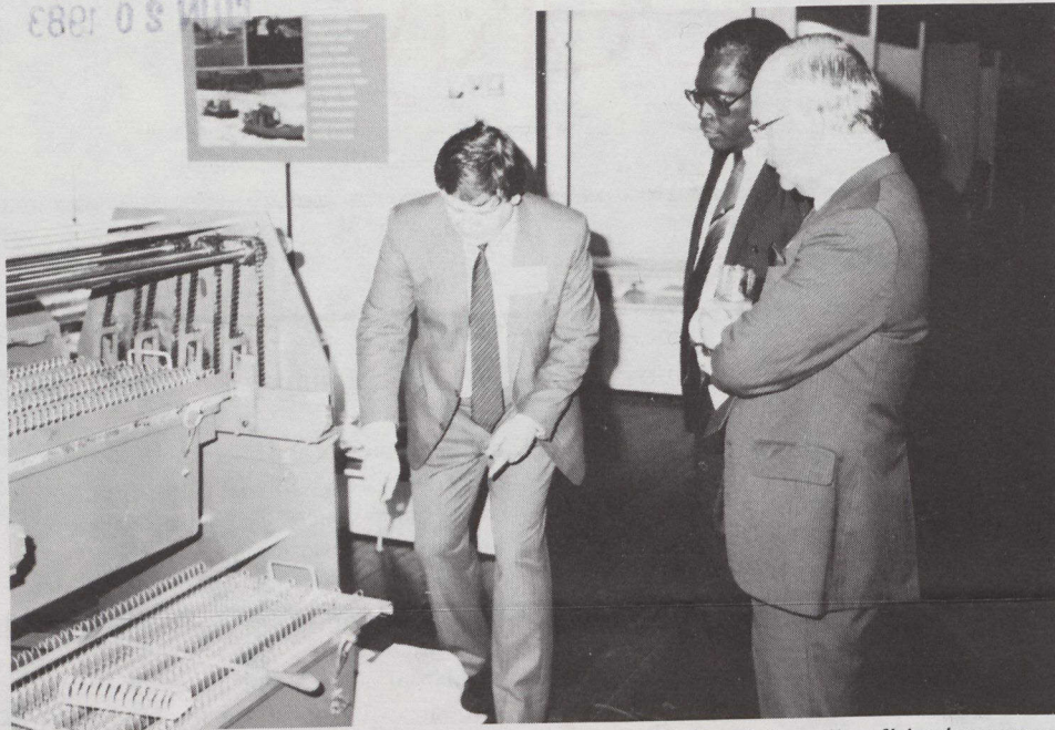
Fisheries division director John Foster demonstrates his firm's long-line fisheries system, the gangbaiter, which baits 320 hooks in record time while cutting bait and double hooking in one operation.
